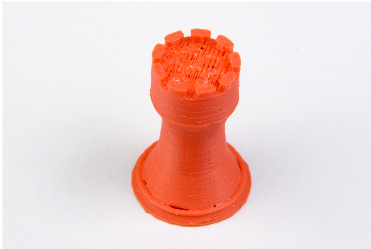
Figure 5.15: An example of insufficient top layers.
