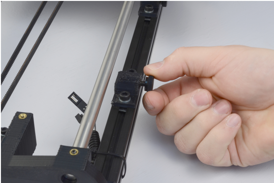
Figure 1.3: Remove the four Y axis bolts
