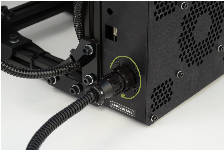
Figure 1.17: The power supply plug correctly plugged in
