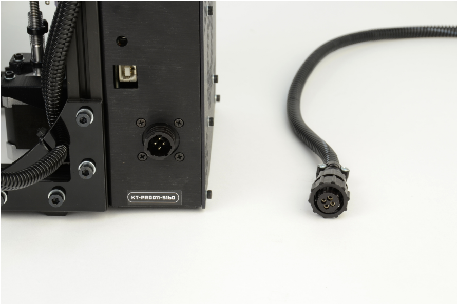
Figure 1.16: 12V DC Power supply plug and receptacle
