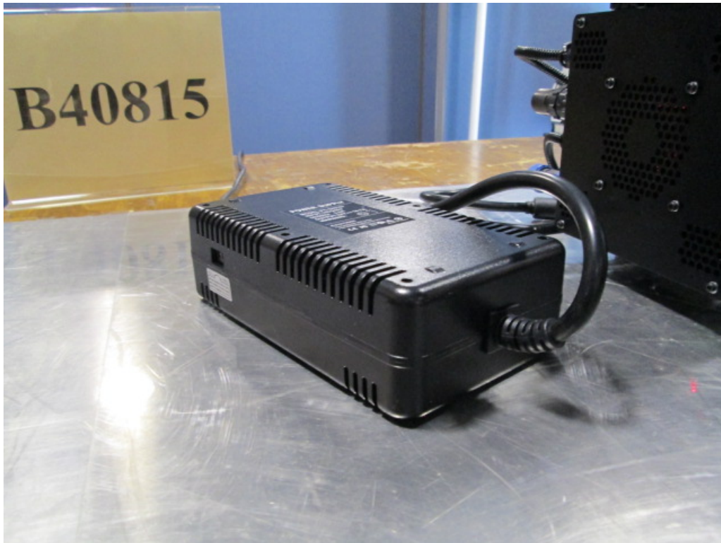
Figure A9. Electrostatic Discharge Test Setup.
