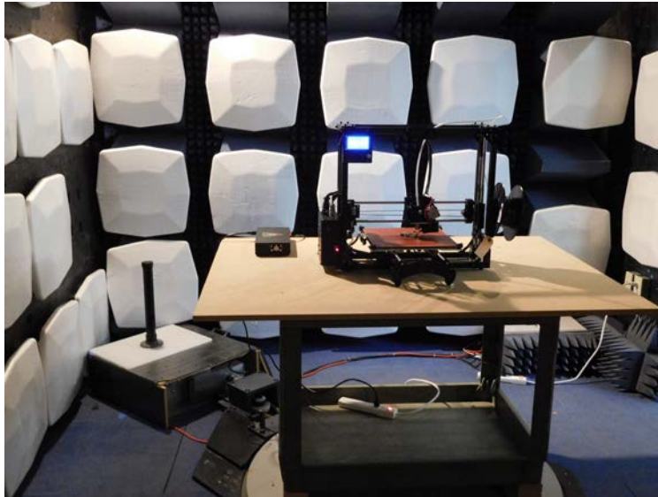
Radiated emissions test setup – printing from SD Card
