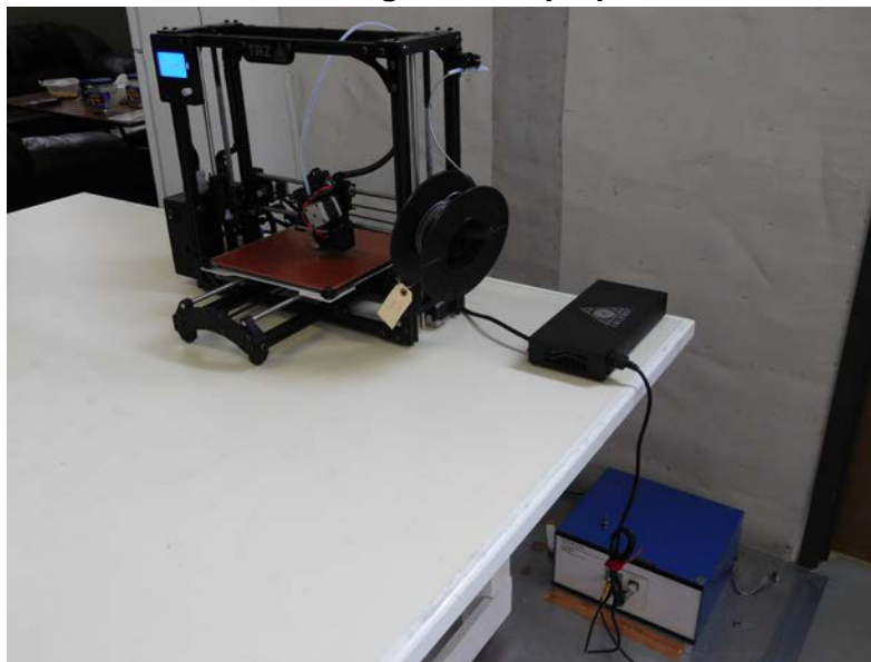
Conducted emissions test setup
