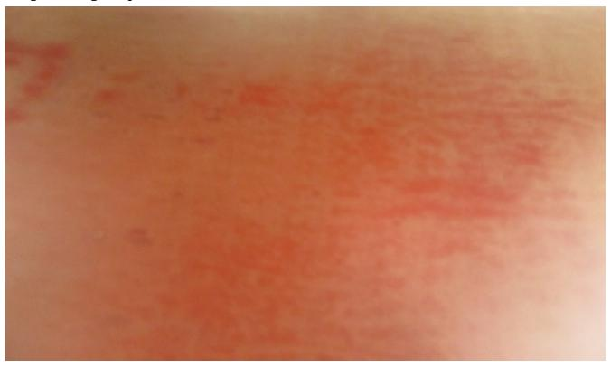
• Some heat pads may fully separate from the glass, see image below. Reject these beds if any fo the delaminated areas are greater than 1/2" in size.
