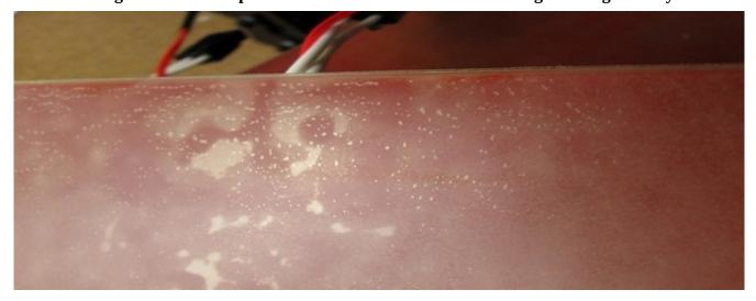
Example of a passable amount of silvering. Note that the silvering is within 2" of the edge and that none of the bubbles are joining together.
