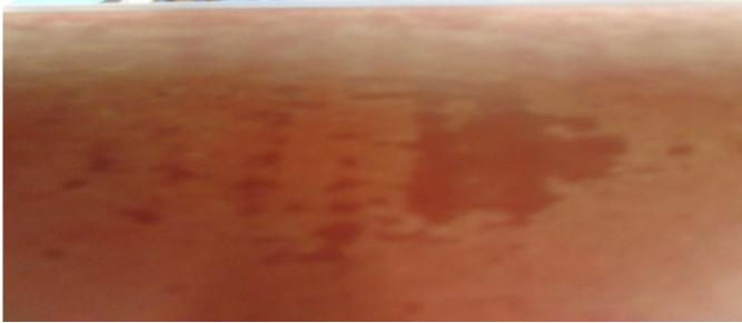
• All heat pads will have some air pockets above the connector on the edge of the bed.
