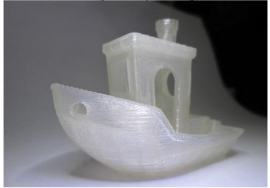
BELOW: Standard PLA settings with min layer time changed from 20 to 40s.
