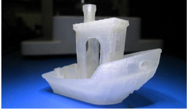
ABOVE: Print with standard PLA settings, you can see a noticeable improvement when the minimum layer setting cuts in, slowing down the print.
