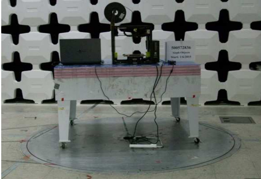
Test Setup – Rear (30 MHz - 4000 MHz)
